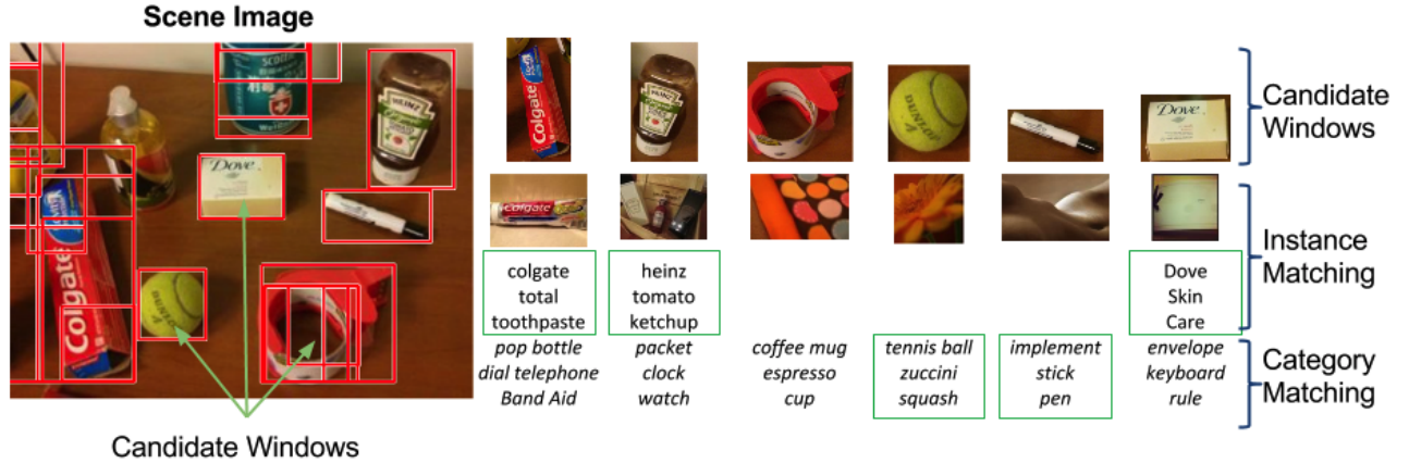
Fig. 3. Instance and category information are often complementary. The image on the left is overlaid with candidate image windows, computed using the selective search method of Uijlings et al. (2013) . Extracted regions are shown on the top row. Below each region is the image that was the best match found by a web-scale instance search. Text below this matching image shows the corresponding instance-level projection; text below that (in italics ) shows the category-level projection derived from Deep Convolutional Imagenet Classifiers (DECAF) ( \phi_{DEC} ). In this example the instance-level projection would likely be able to resolve 3 of 6 objects for typical user queries in this scene (ketchup, toothpaste, bar of soap), while the category-level projection could likely resolve 2 of 6 (ball, pen). The liquid soap container was missed by the selective search in this example but is reasonably likely to have been recognized as a bottle by the DECAF models.
